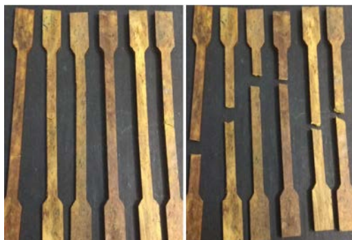
Fig.7 (a) tensile strength specimen (b) After tensile strength testing
