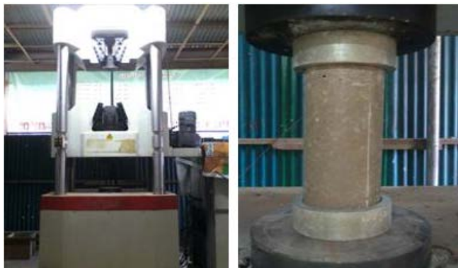
Fig. 2 Compression test set up (Ernesto J. Guades et al. , 2016)
