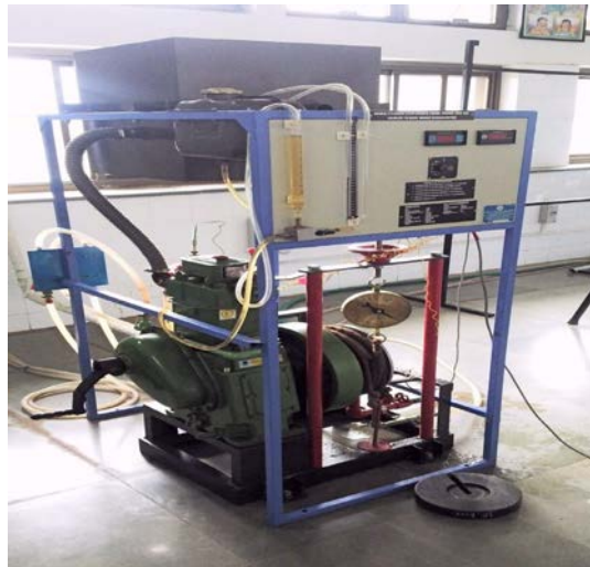
Fig.1 Hydraulic dynamometer, measuring equipment
