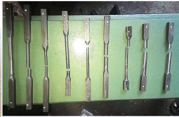
Fig. 2 Mild steel Specimens after failure
