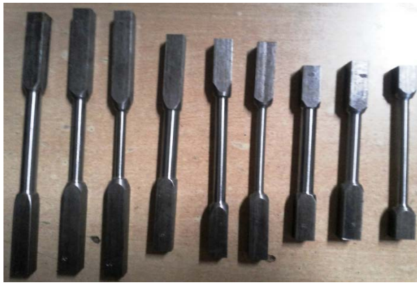
Fig. 1 Mild steel Specimens before failure
