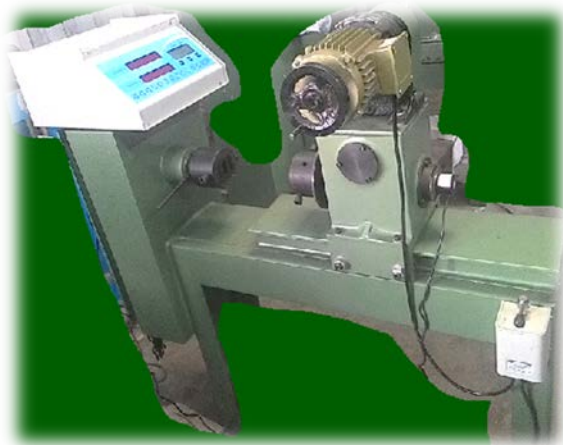
Fig. 3 Digital torsion testing machine 200N-m
