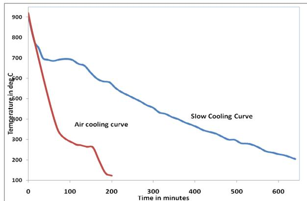
Fig.1 Temperature profile of slow cooled and air cooled bars
