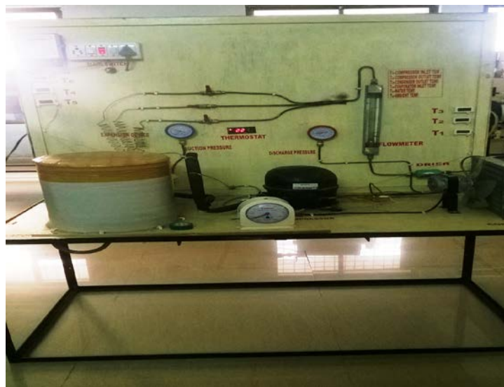
Fig. 3The apparatus consist of a domestic refrigerator
