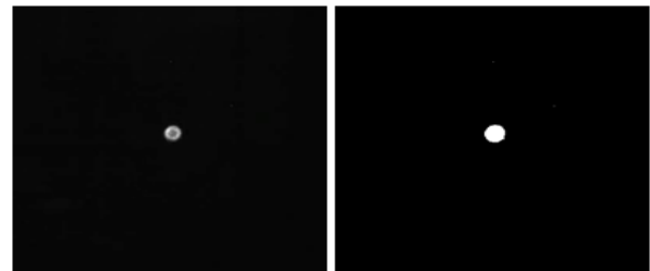
Fig.14 Comparison of the static blob (left image) and its thresholded bitmask (right image)
