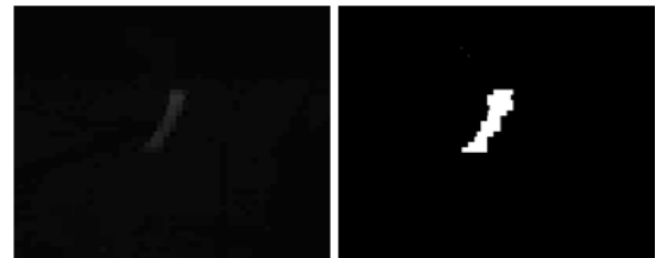
Fig.15 Comparison of the blurred blob (left image) and its threshold bitmask (right image)
