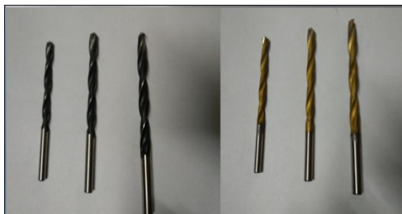
Fig. 2 Simple HSS and TiN coated HSS twist drill
