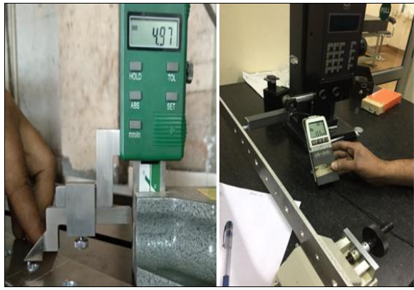
Fig. 5 Measurements of burr height and surface roughness
