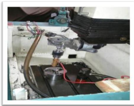
Fig. 2 Experimental setup: The automatic ELEKTRAPLUS PS 20 (T-3822) machine with mechanism of the rotational tool
