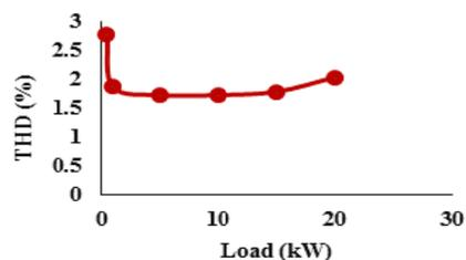
Fig 9. Load changes versus load current THD
