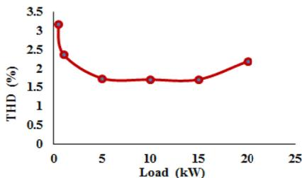
Fig 8. Load changes versus load voltage THD
