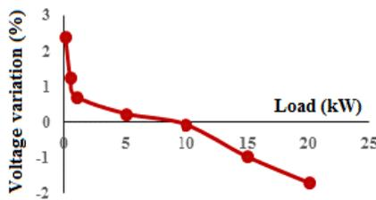
Fig 7. Load changes versus % voltage variation
