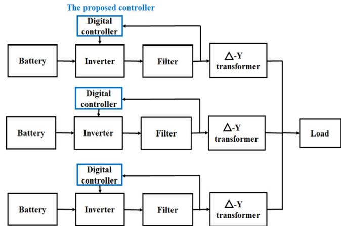
Fig 1. Block diagram of the proposed model
