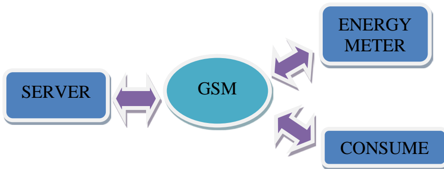
Fig.2 Overview of the prepaid metering system
