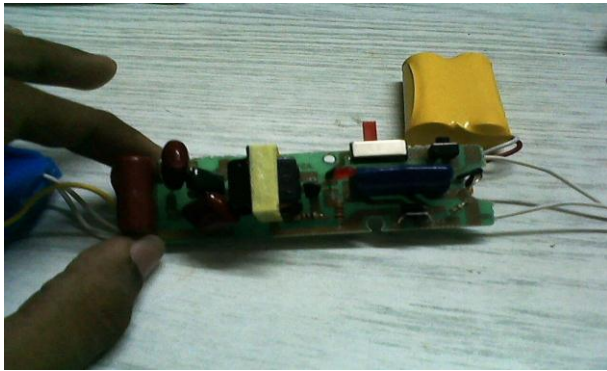
Fig. 7 Input control circuit for safe operation of Tesla coil circuit
