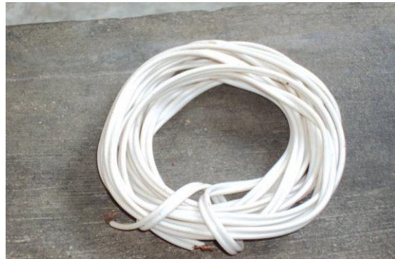
Fig. 5 Radio frequency insulated wire for fabrication of primary winding
