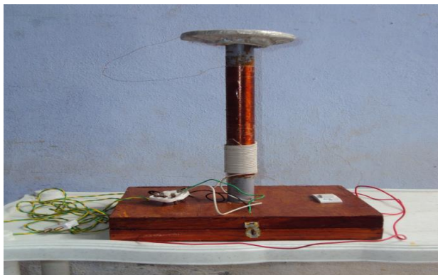
Fig. 8 Tesla Coil with L_1 & L_2 wound surrounding the insulator former without resistance potential divider
