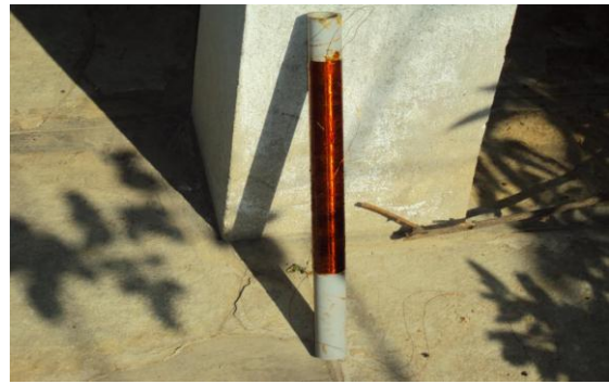
Fig. 4 Completion of Winding L_2 on insulation former
