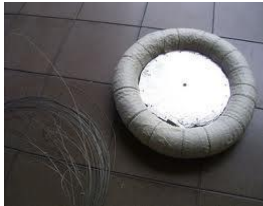
Fig. 6 Fabrication of toroid with aluminum foils.
