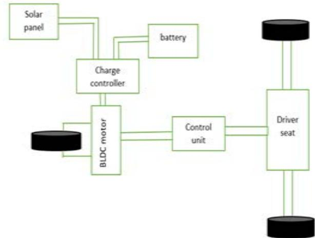
Fig. 1 Block diagram of the proposed model
