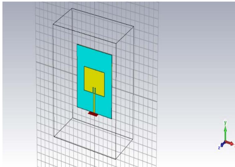
Fig. 4 Structure of Handbag in zipper antenna
