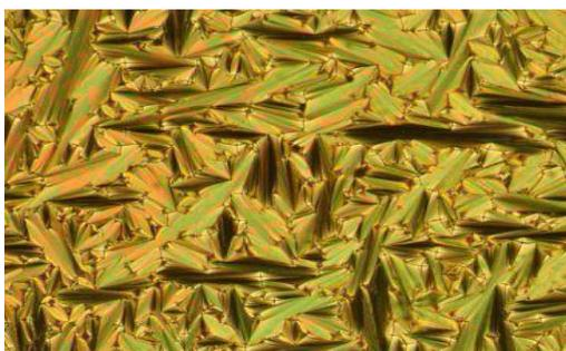
Fig. 2 Focal Conic Fan Shaped Texture of Smectic-A Phase
