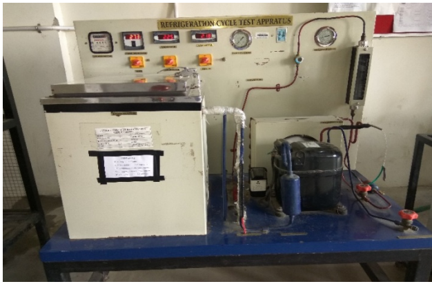
Fig.1 Vapour Compression Test Rig
