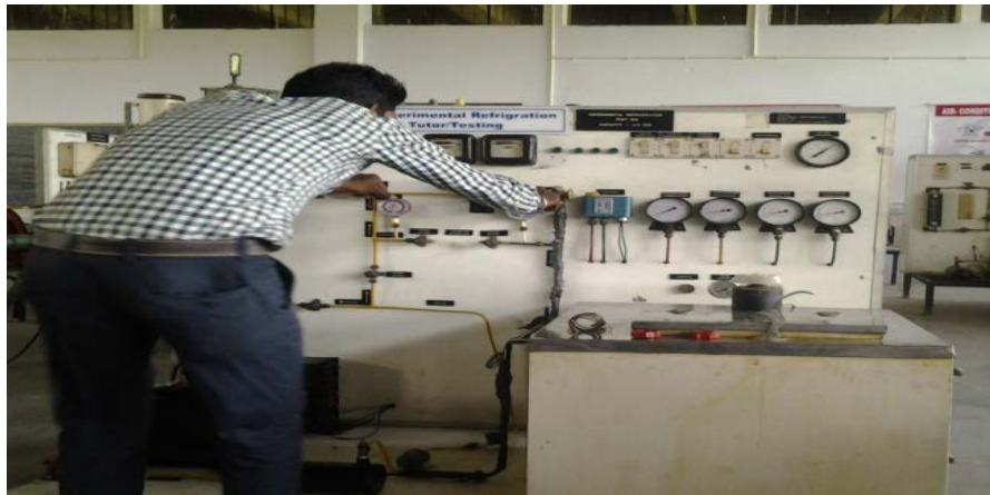
Fig.8 Installation of Pressure Guages
