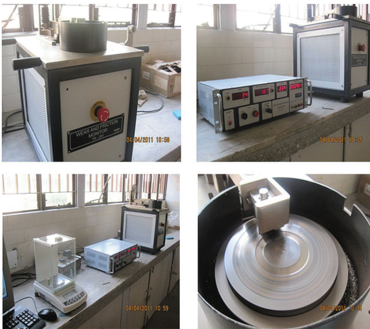
Fig. 2 Wear Testing Apparatus as per ASTM G99 standards
