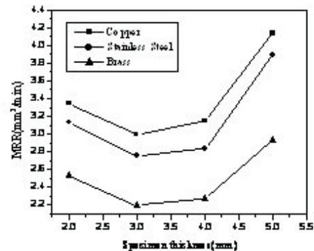
Fig. 4 Effect of specimen thickness on MRR
