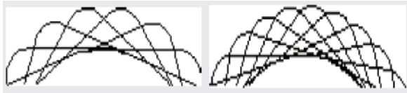
Fig.7 Pulsating action of flat faced tools [14]
