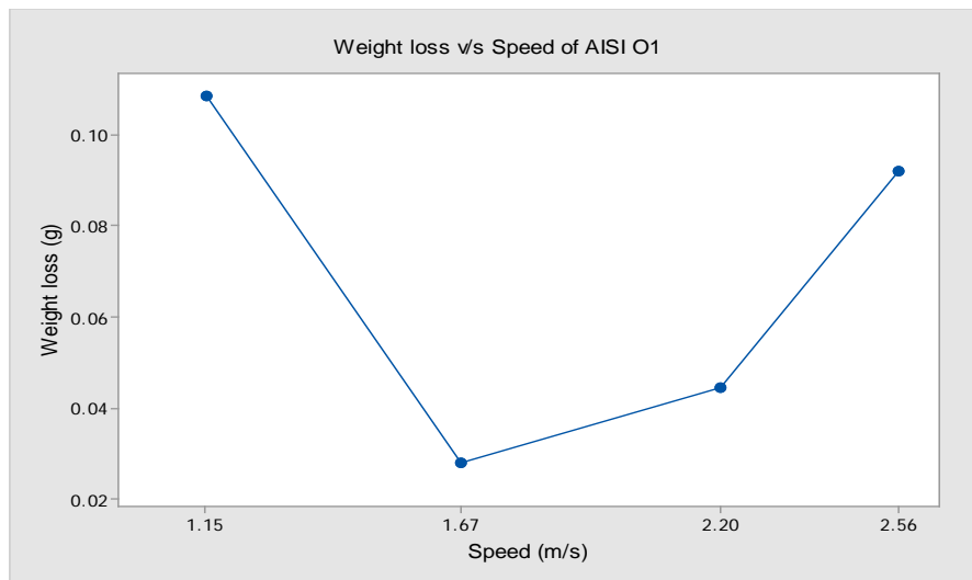
Fig.2 Weight loss vs speed AISI O1
