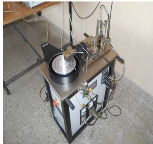
Fig.2 Wear and friction measuring test rig TR-2
