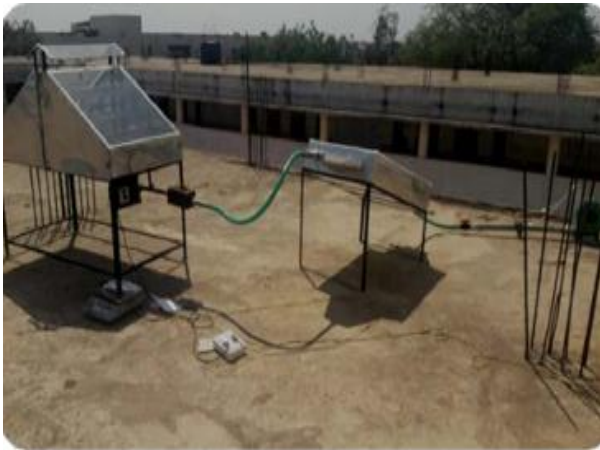
Fig. 6 Mixed mode forced convection solar dryer
