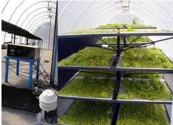
Fig. 1 Tunnel type solar dryer
