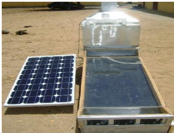
Fig. 4 Indirect mode solar dryer
