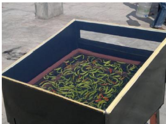
Fig. 2 Box type solar dryer
