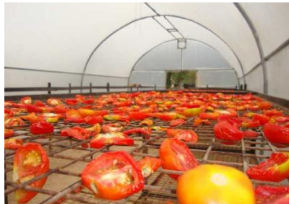
Fig. 5 Tunnel type solar dryer
