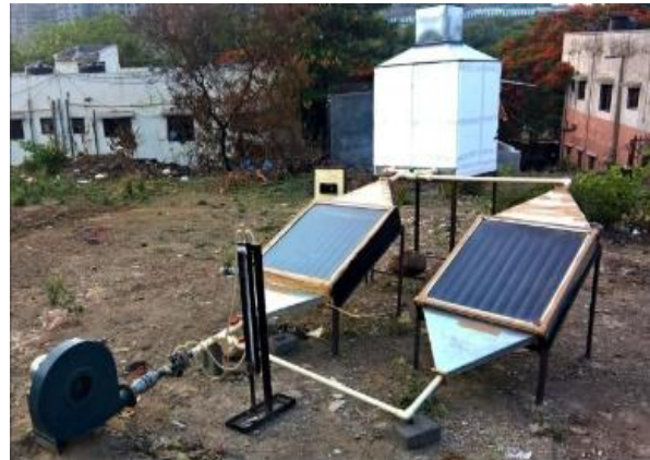
Fig. 3 Indirect mode forced convection solar dryer
