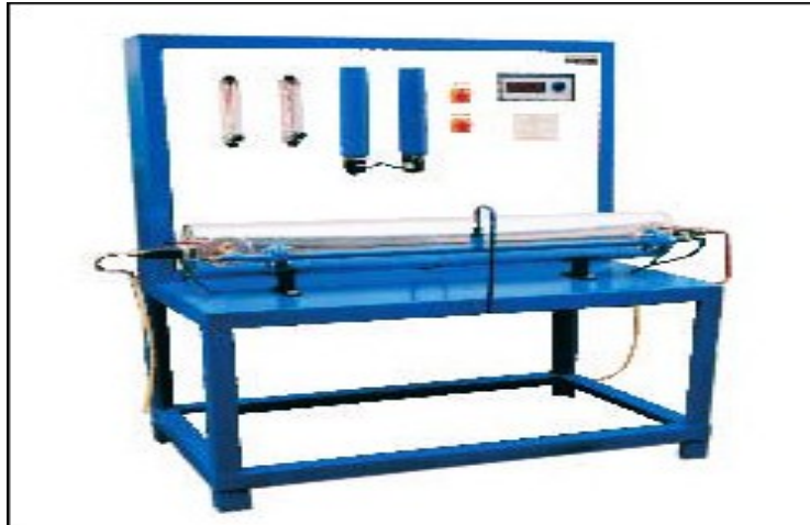
Fig. 1 Experimental setup of the double pipe heat exchanger
