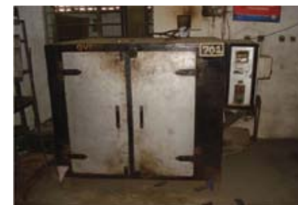
Fig 2.4 Post Curing Oven. The Cured components have to be kept inside For 8 Hrs
