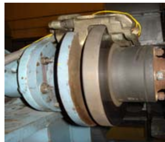
Fig 4.3(b) Inertia Brake Dynamometer Setup for testing Brake Performance
