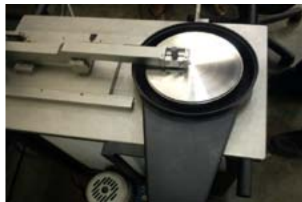
Fig. 4.1 (B) Pin on disc apparatus
