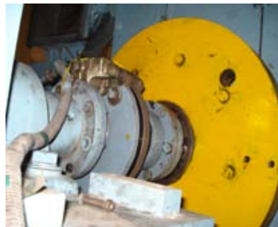
Fig 4.3(a). Disc Brake Assembly & Caliper
