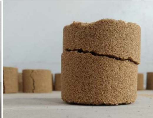
Fig. 4 a) Universal sand strength machine in compression mode, b) Compression tested specimen
