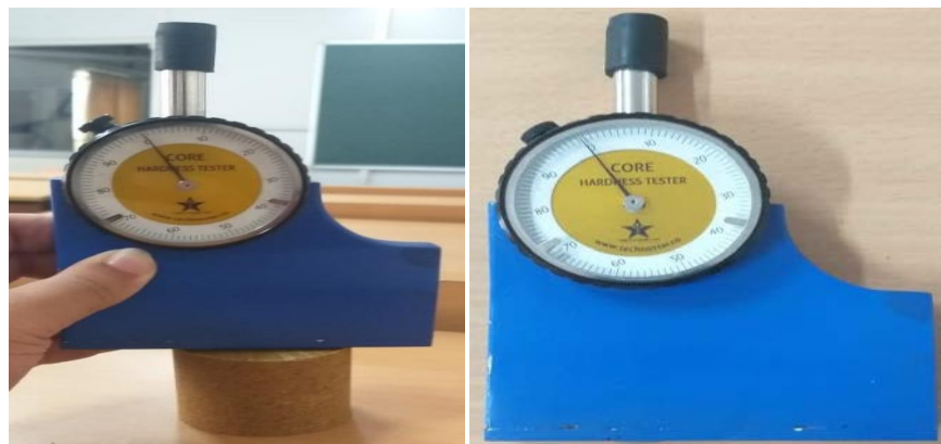
Fig. 7 a) Hardness tester, b) Measuring mould hardness
