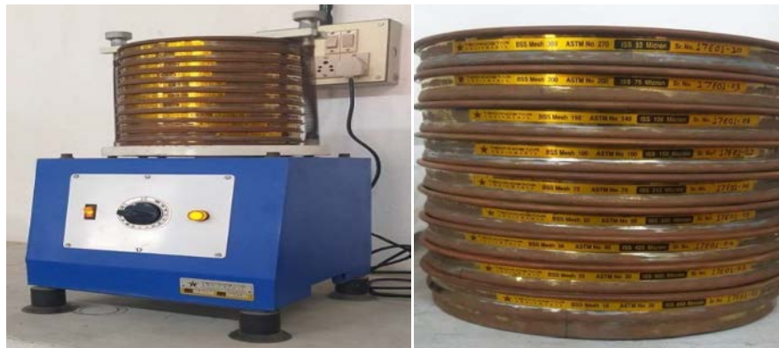
Fig 2 a) Sieve shaker, b) Arrangement of sieves
