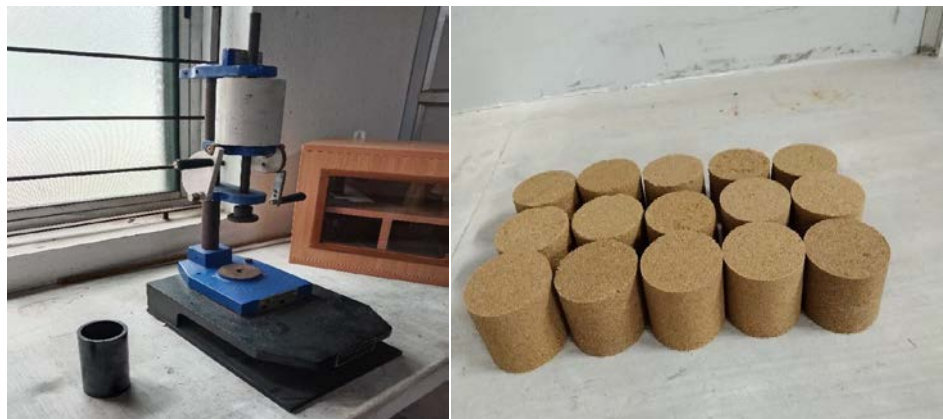
Fig. 3 a) Sand rammer equipment b) Fabrication of 15 standard samples
