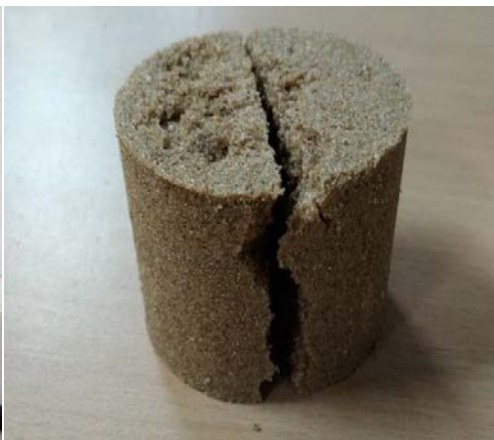
Fig. 5 a) Universal sand strength machine in shear mode, b) Shear tested specimen
