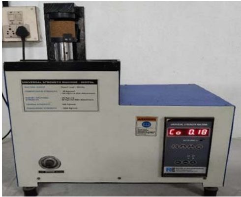
Fig. 4 a) Universal sand strength machine in compression mode, b) Compression tested specimen
