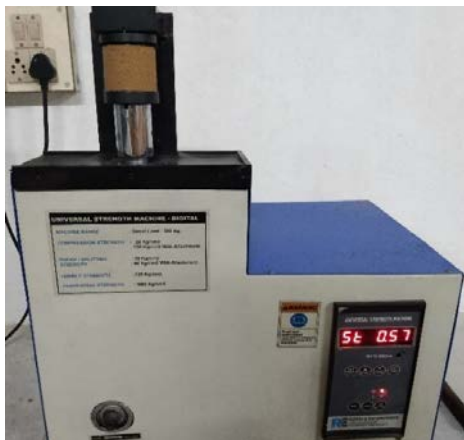
Fig. 5 a) Universal sand strength machine in shear mode, b) Shear tested specimen
