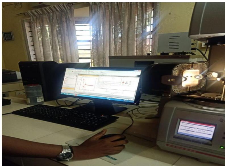
Fig. 3 Viscosity measurement of Al 2 O 3 and CuO nanofluid samples
